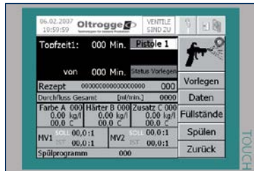
Siemens Simatic Panel
